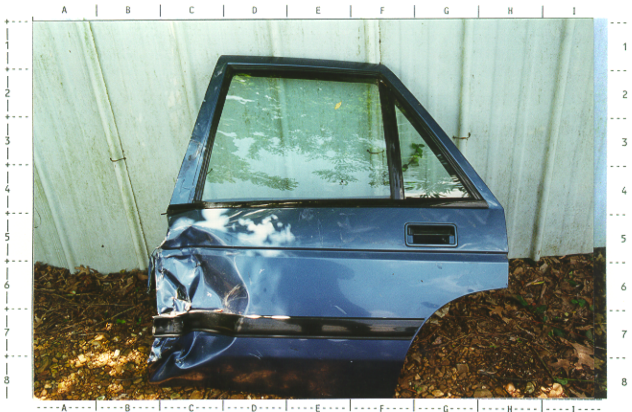
# 50 -- Damage to left rear door of 1991 Chevrolet Corsica; NOTE: door was removed during extraction process
